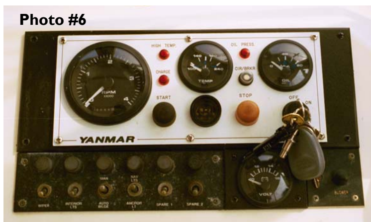
← Helm gauges and DC switches and fuses.
